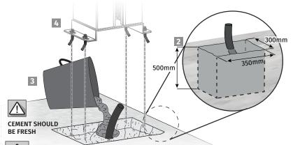
For the correct functioning of the automatism, it is necessary to take into the dimensions mentioned in the image. Leave a 200mm free space on the door side of each automatism, so you can open the automatism door whenever necessary.
